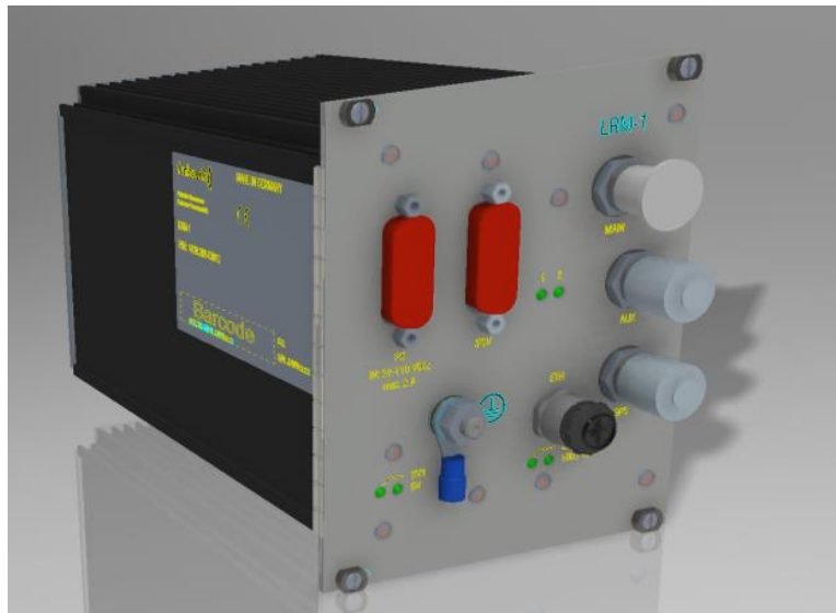
Figure 12 - RCDPS Prototype (case for installation in rack of Bombardier TU's)
